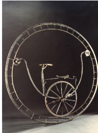
Figure 1.1: One-Wheel Vehicle (Rousseau-Workshops, France, wheel radius 2 m, without steer, 1869)
